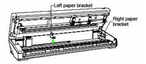
Insert the paper roll into the left and right paper brackets. Be sure to insert the roll so the end of the paper comes out from underneath the roll, as shown below.
