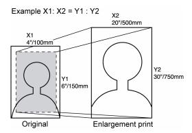
The area of the original that can be enlarged is illustrated below. Refer to the next page for information on highlighting the area you want to enlarge using a command sheet.
