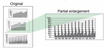
The width of the area you highlight on the command sheet becomes the width of the printed enlargement. The length expands according to the enlargement ratio of the print width.
