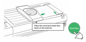
A "Scanning" message appears in the display while the printer scans the command sheet. When it is finished, the Original screen is displayed.
