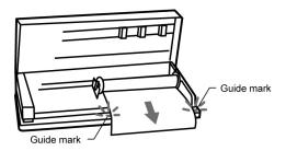
Before printing, verify that the printer cover is properly closed by pushing down on BOTH SIDES until it locks into place. If both sides of the cover are not closed, only part of your poster will print.
