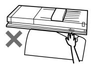
Avoid contact with the thermal heads (which retain heat) immediately after using the printer.
