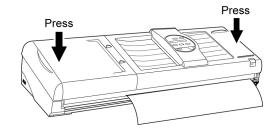
Avoid pressing down on the printer or scanner cover while the printer is in operation.
